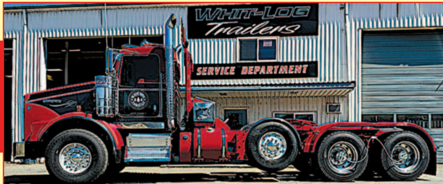
Black Rock Timber, DALLAS, OR, Brand Whit-Log CUSTOM Lowboy Truck Equipment. Custom Steel Cab Rack, Custom Aluminum Hydraulic Tank/Toolbox Combo, Frame Mount Air/Electric/Hydraulic Station, Custom Whit-Log HD Slider, Minimizer Fenders, Custom Tail Section, Custom Cab Accessories (Cab Lights, Horns, Air Cleaner Lights, Visor, Etc.), Custom "Pull Me Over Red" Paint, and Much More... Thanks Ross!
