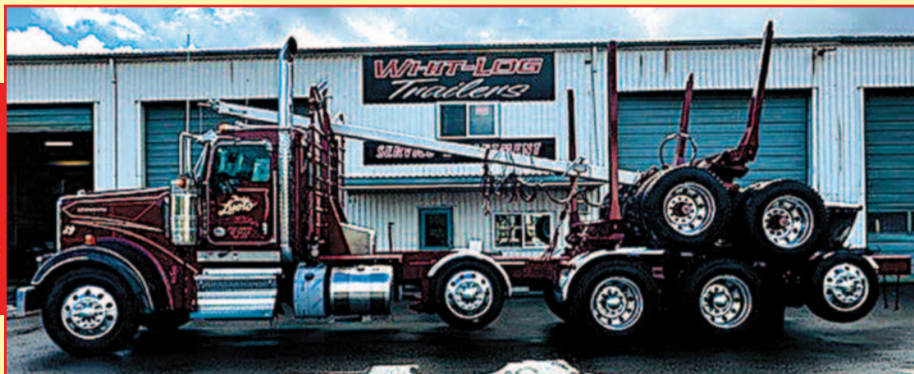
Randy Luoto Trucking LLC, CARLTON, OR, Brand New Whit-Log SEWC100 Long Logger (Bendix Disc Brakes) & Matching Truck Equipment. Vulcan Scales, Custom Aluminum Cab Rack, 88" Truck Bunk w/ Trailer Bolster, Pipe Ride Assembly for Riding Trailer Behind Bunk, Aluminum Fenders, Chrome Light Bars, Custom "Radiant Fire Pearl" Paint, and Much More... Thanks Randy!
